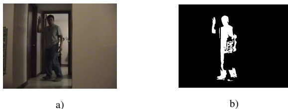
Figure 9 Object Detection Results for an Indoor Scene, a) Image Containing Moving Object, b) Foreground Mask Obtained Using a 3 \times 3 Window
