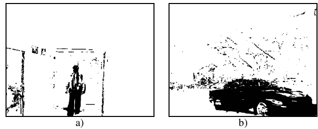
Figure 5. Results obtained using Simulink. a) Threshold value 0.6 for indoor scene, b) Threshold value 0.6 for outdoor scene.
