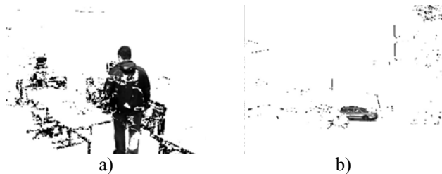
Figure 9. Results obtained using Simulink, a) Threshold value 0.85 for indoor scene, b) Threshold value 0.2 for outdoor scene.
